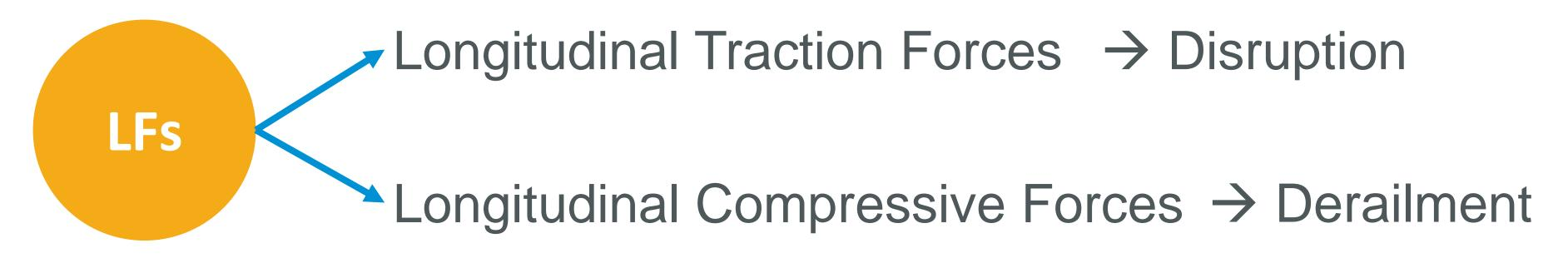
LCFs can cause a derailment when, depending on track geometry, they are over the acceptable value (**permissible LCF**) even just for one of the wagons
